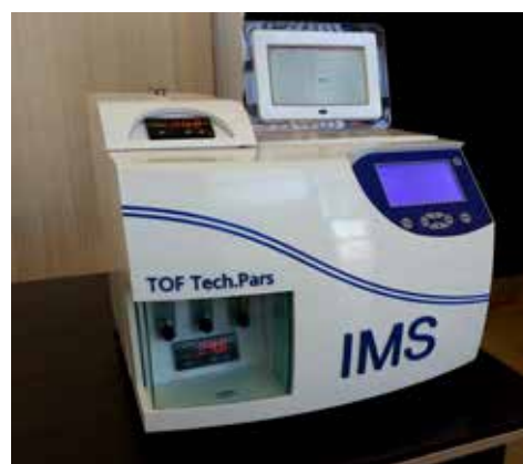
Two Types of Ion Mobility Mass Spectrometer Constructed in the Department of Chemistry
